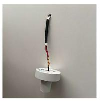
3. Put a length of heatshrink on the fixed installation cable. Connect the crimp connectors to the fixed installation cable.
