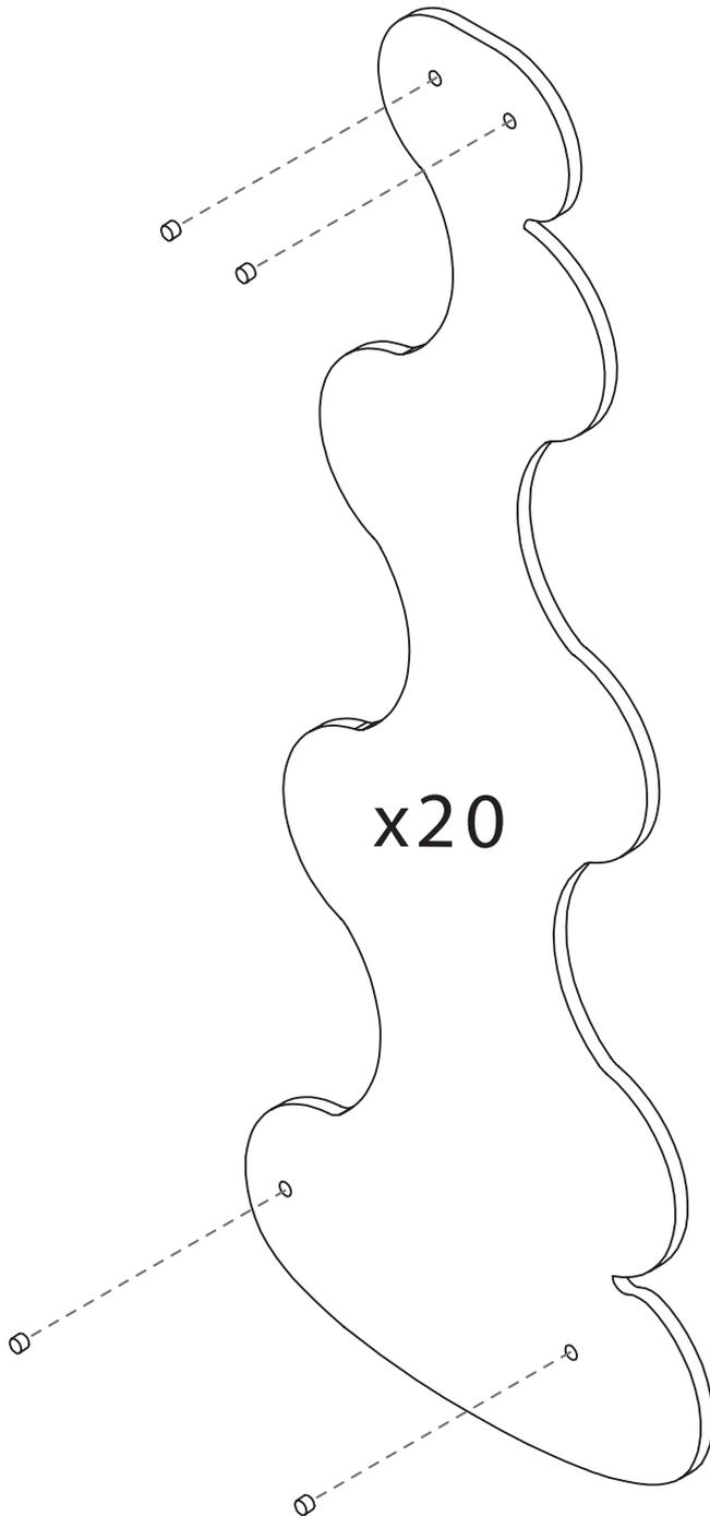
Push out the 4 plugs per panel to make way for the plastic clips.
