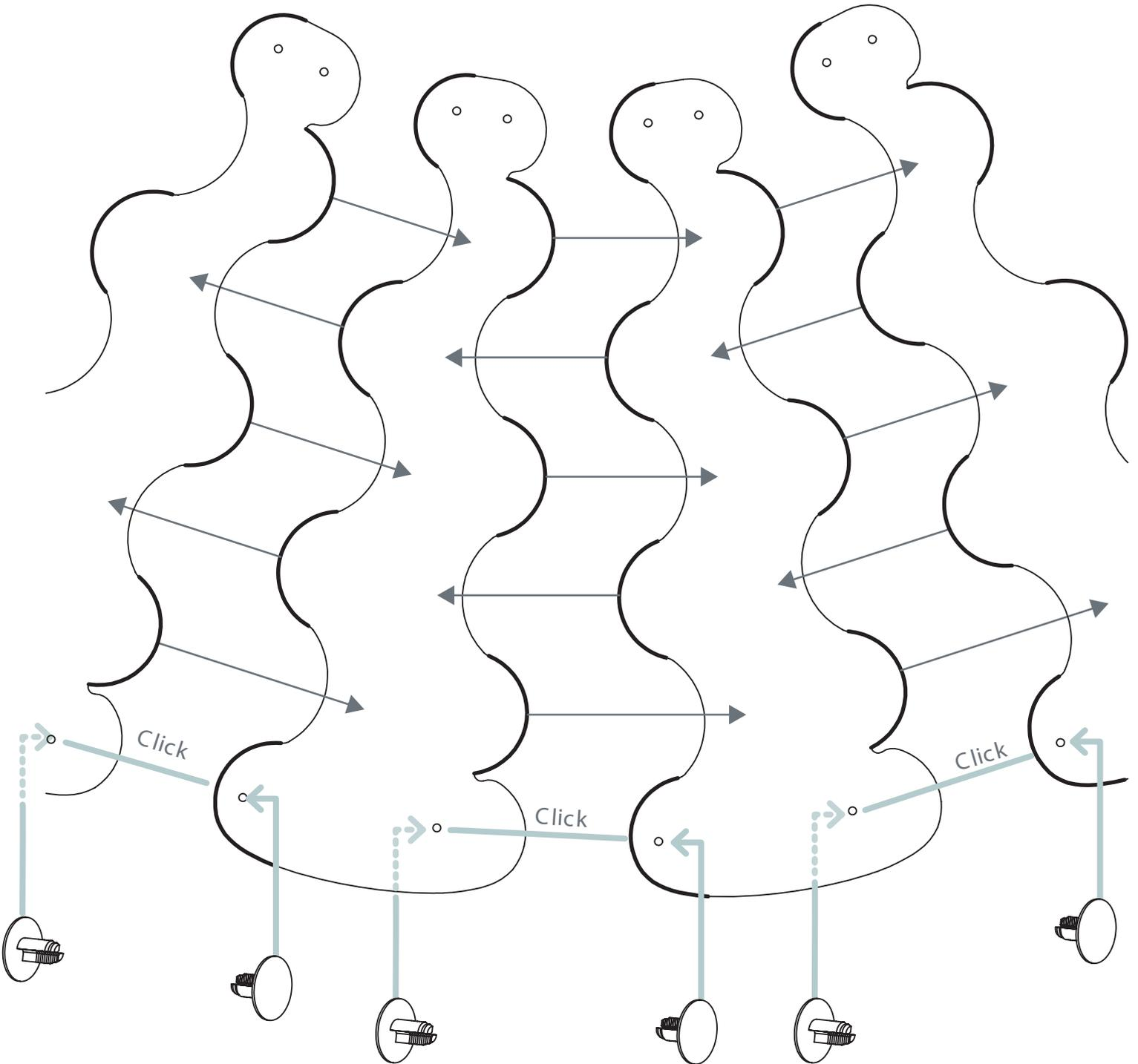
Once two panels are woven together, use two of the shorter Ratchet Rivets (13 mm) to lock them together.
