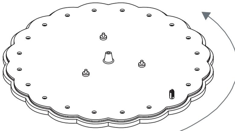
Insert Large Ratchet Rivets (19mm) in all holes around edge.
